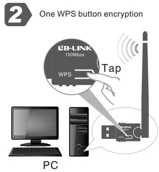
Note: Press router's WPS button, then press adapter's WPS button in 5 seconds until the adapter's led light is flashing
